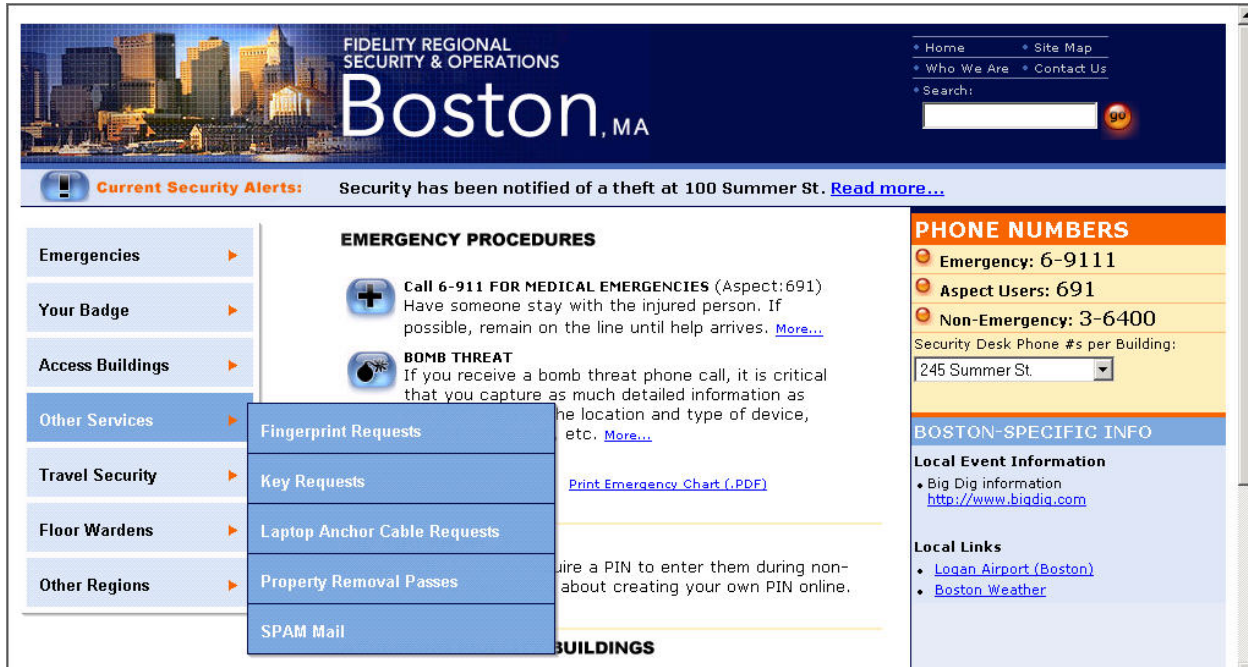
Figure 6. Fly-out Menu. On mouseover, these menus open automatically, and sub-items are selectable. We have seen usability issues with this type of menu, when users attempt to select a sub-menu item and mistakenly move the mouse over another menu item, thereby losing the fly-out they originally wanted. This is often called the “diagonal problem”.
